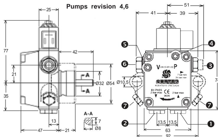
Inlet ① and Return ② with direct sealing for revision 5 and 6 models (sealing with washers can also be used)
